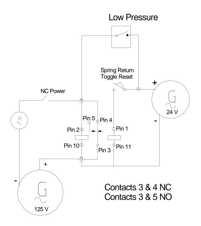
When Low Pressure Switch closes, relay sets to contacts 3 & 5, removing power from motor. To reset must close spring return toggle switch to return relay to contacts 3 & 4 and restore power to motor.
