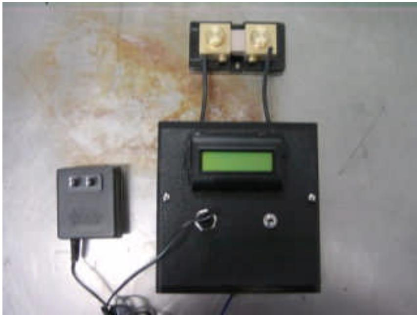
This modification is suitable for applications < 60 VDC and ~ 350 Amps. If a higher voltage is in use, then a voltage divider can be installed on the voltage sense line to reduce the voltage to the meter to less than 60 VDC. The output then will be multiplied by the corresponding voltage divider factor, e.g., if divide the voltage in half, then the output is multiplied by 20, 10X for the shunt and 2X for the voltage divider.
