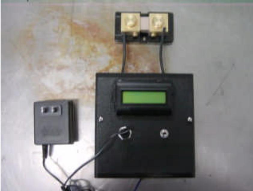
This modification is suitable for applications  $< 60$  VDC and  $\sim 350$  Amps. If a higher voltage is in use, then a voltage divider can be installed on the voltage sense line to reduce the voltage to the meter to less than 60 VDC. The output then will be multiplied by the corresponding voltage divider factor, e.g., if divide the voltage in half, then the output is multiplied by 20, 10X for the shunt and 2X for the voltage divider.
